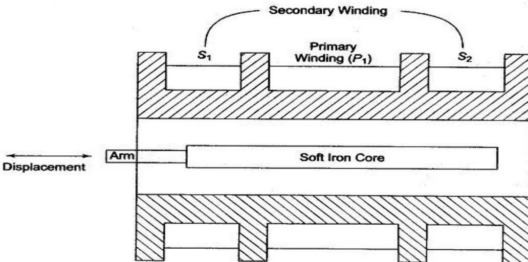
**Fig. 13.19** Construction of a Linear Variable Differential Transducer (LVDT)
