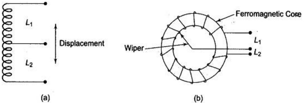
**Fig. 13.17** (a) Linear Differential Output Transducer
