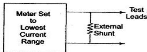
**Fig. 3.5** Extending of Ammeters
