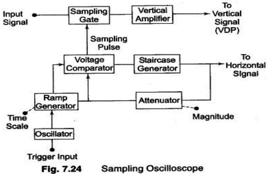
Figure 7.24 shows a block diagram of a sampling oscilloscope. The input waveform is applied to the sampling gate. The input waveform is sampled whenever a sampling pulse opens the sampling gate. The sampling must be synchronized with the input signal frequency. The signal is delayed in the vertical amplifier, allowing the horizontal sweep to be initiated by the input signal. The waveforms are shown in Fig. 7.25.
