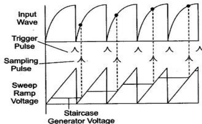
**Fig. 7.25 Various Waveforms at Each Block of a Sampling Oscilloscope**
