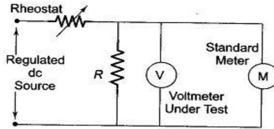
**Fig. 4.32** Calibration of Voltmeter
