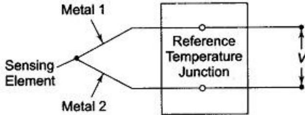
**Fig. 13.41** Basic Thermocouple Connection
