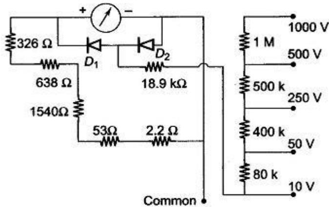
**Fig. 4.37** AC Voltmeter Section of a Multimeter
