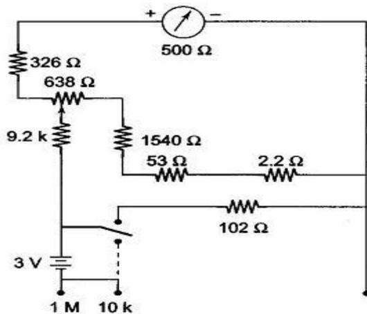
**Fig. 4.38** Ohmmeter Section of a Multimeter
