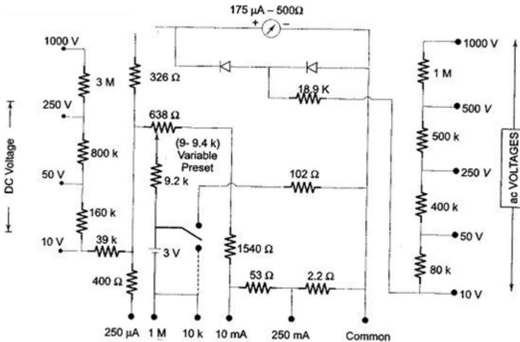
**Diagram of a Multimeter**
