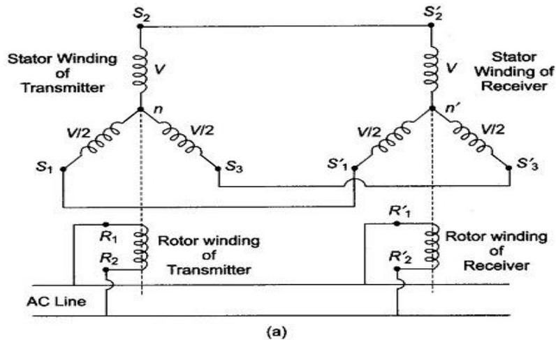
(a) Torque Transmission Using Synchro Trans
