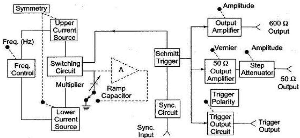
**Fig. Block Diagram of a Pulse Generator**
