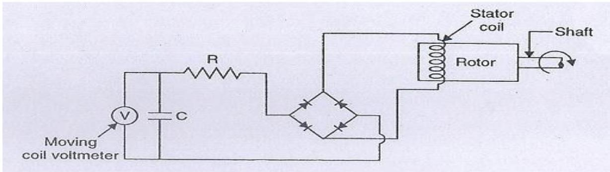
It consists of, like an alternator, a stationary armature (stator) and a rotating field system (rotor). Owing to the generation of e.m.f in a stationary coil on a stator, commutation problems no longer exist. The alternating e.m.f. induced in the stationary coil is rectified, and the output D.C. voltage is measured with the help of a moving coil voltmeter (V).
