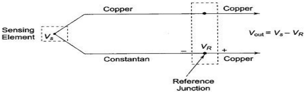
**Fig. 13.44** A Type T Thermocouple with Reference Junction
