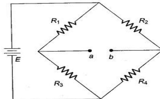
**Fig. 11.2** Unbalanced Wheatstone's Bridge
