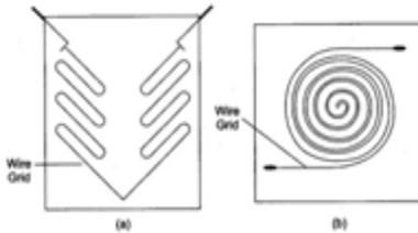
**Fig. 13.8** (a) and (c) Torque Type Gauge (b) Helical Gauge
