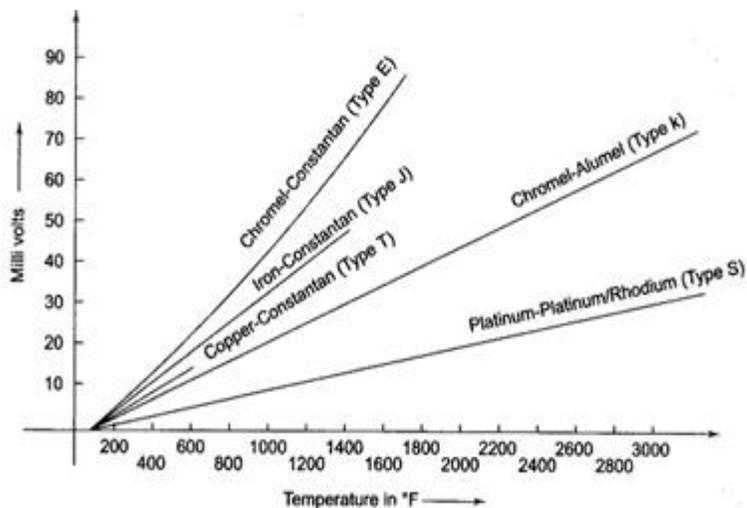
Fig. 13.43 Thermocouple Output Voltage as a Function of Temperature for Various Thermocouple materials
