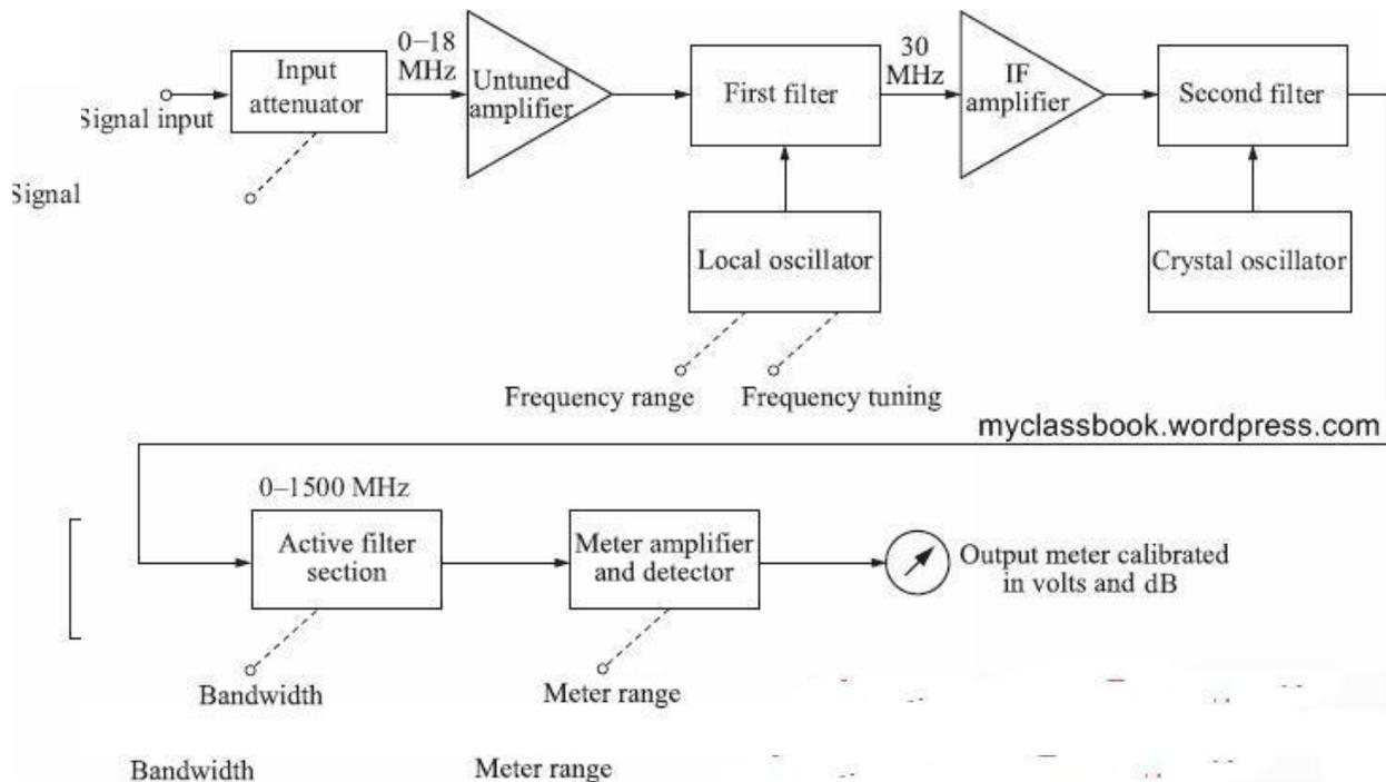
The block schematic of the wave analyzer using the heterodyning principle is shown in fig. above. The operating frequency range of this instrument is from 10 kHz to 18 MHz in 18 overlapping bands selected by the frequency range control of the local oscillator. The bandwidth is controlled by an active filter and can be selected at 200, 1000, and 3000 Hz.
