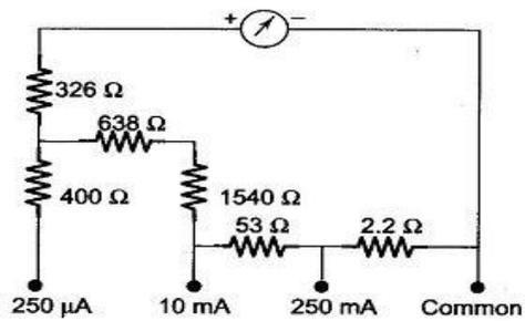
**Fig. 4.35** dc Ammeter Section of a Multimeter
