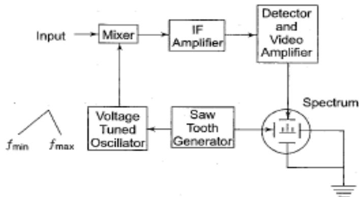
The RF input to be analyzed is applied to the input attenuator. After attenuating, the signal is fed to low pass filter. The low pass filter suppresses high frequency components and allows low frequency components to pass through it. The output of the low pass filter is given to the mixer, where this signal is fixed with the signal coming from voltage controlled or voltage tuned oscillator.
