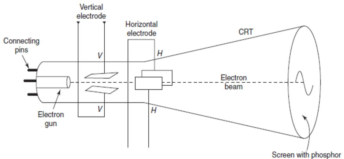
**Figure 14-2** Components of a cathode-ray oscilloscope
