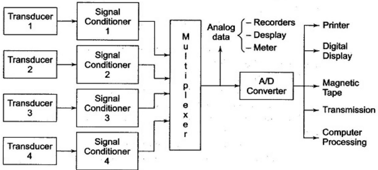
A typical Data Acquisition System consists of individual sensors with the necessary signal conditioning, data conversion, data processing, multiplexing, data handling and associated transmission, storage and display systems.
