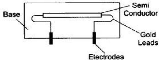
**Fig. 13.10** Semiconductor Strain Gauge
