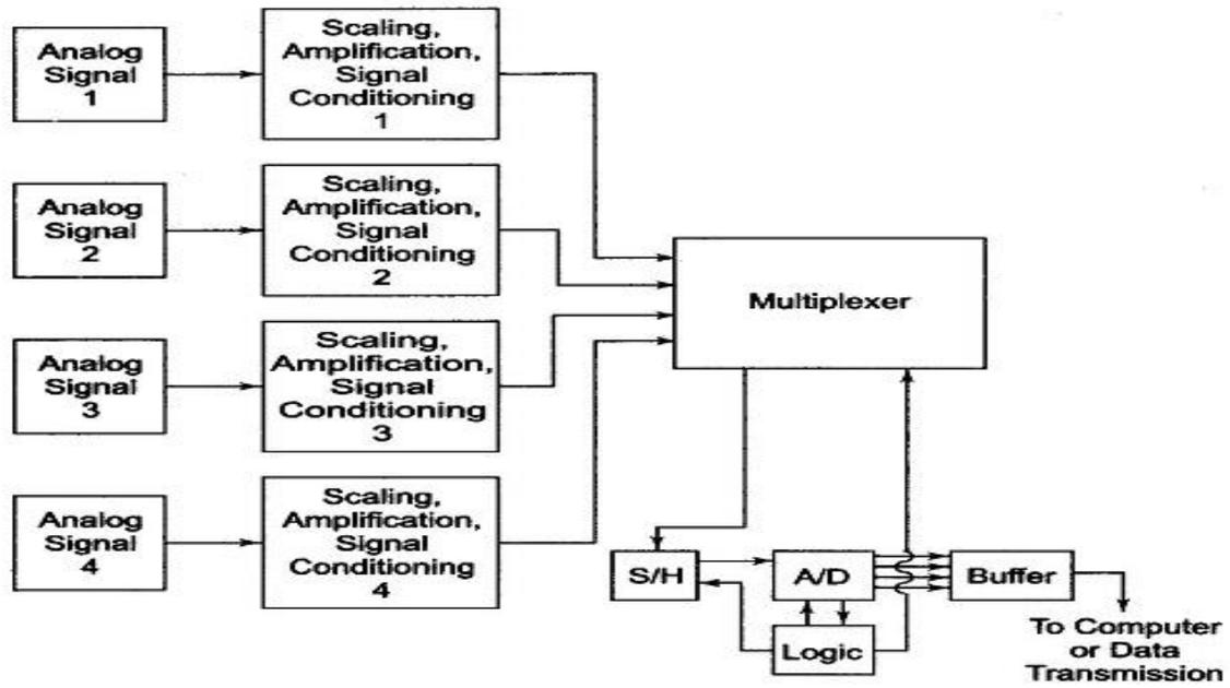
**Fig. 17.5** Multi-channel DAS (A/D Preceded by a Multiplexer)
