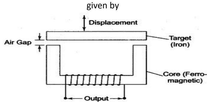
**Fig. 13.16(a)** Variable Reluctance Transducer
