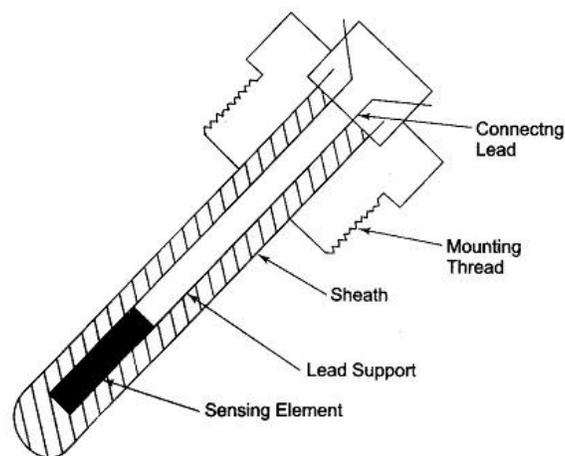
**Fig. 13.40(a)** Industrial Platinum Resistance Thermometer
