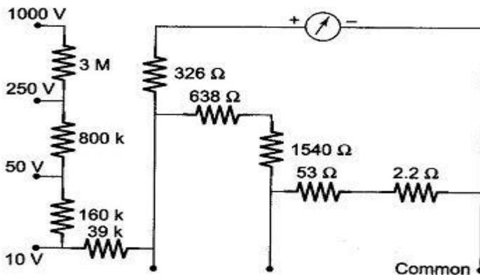
**Fig. 4.36** DC Voltmeter Section of a Multimeter
