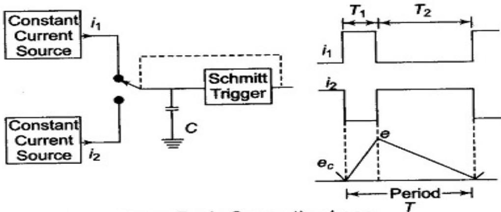
**Fig. Basic Generating Loop**
