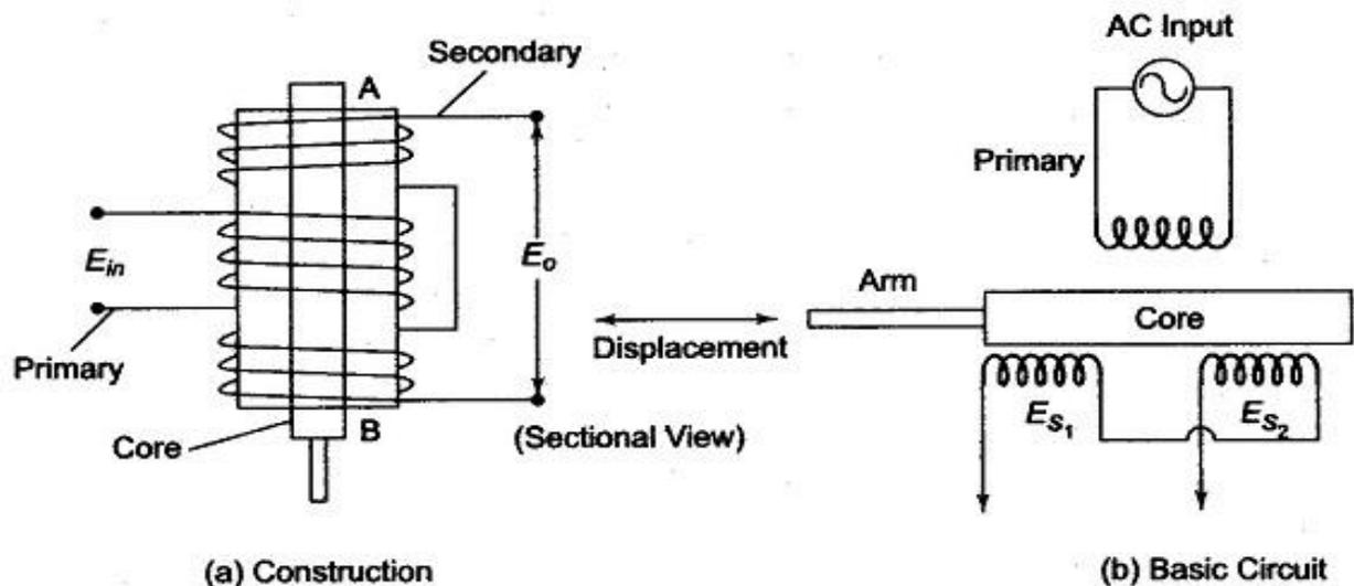
**Fig. 13.20** Secondary Winding Connected for Differential Output
