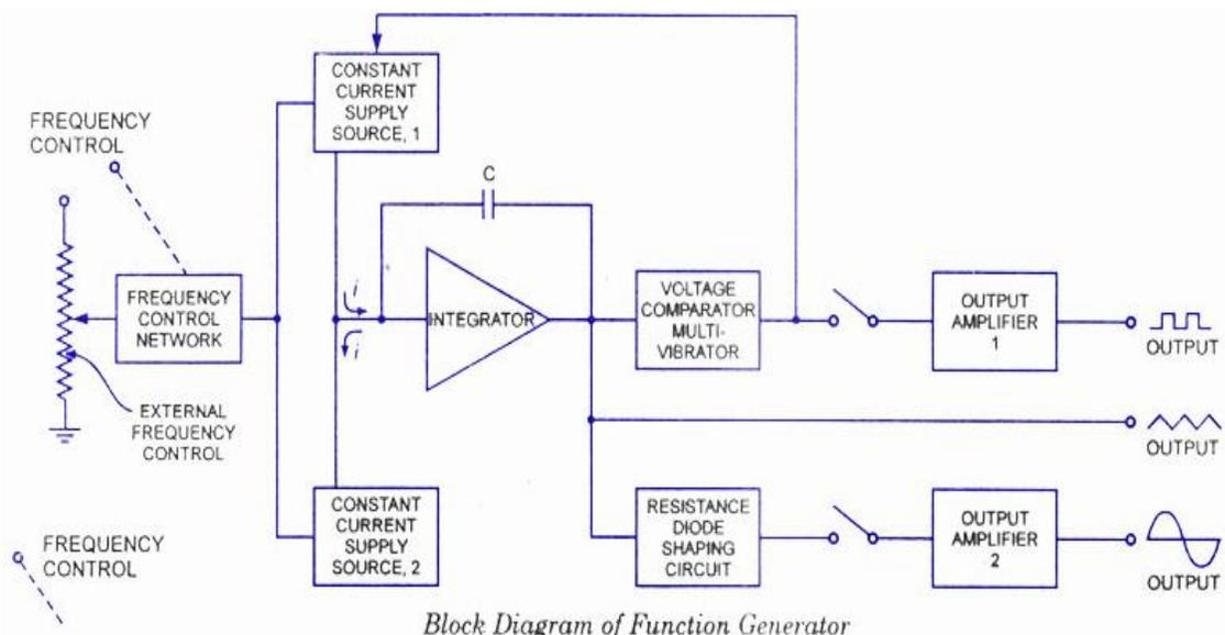
The block diagram of a function generator is illustrated in fig. Usually the frequency is controlled by varying the capacitor in the LC or RC circuit. In the instrument the frequency is controlled by varying the magnitude of current which drives the integrator. The instrument produces sine, triangular and square waves with a frequency range of 0.01 Hz to 100 kHz.
