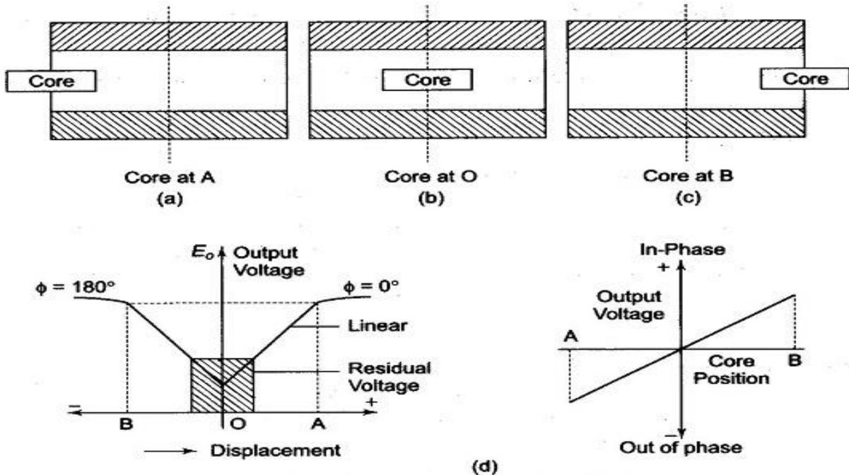
**Fig. 13.21** (a), (b), (c) Various Core Position of LVDT
