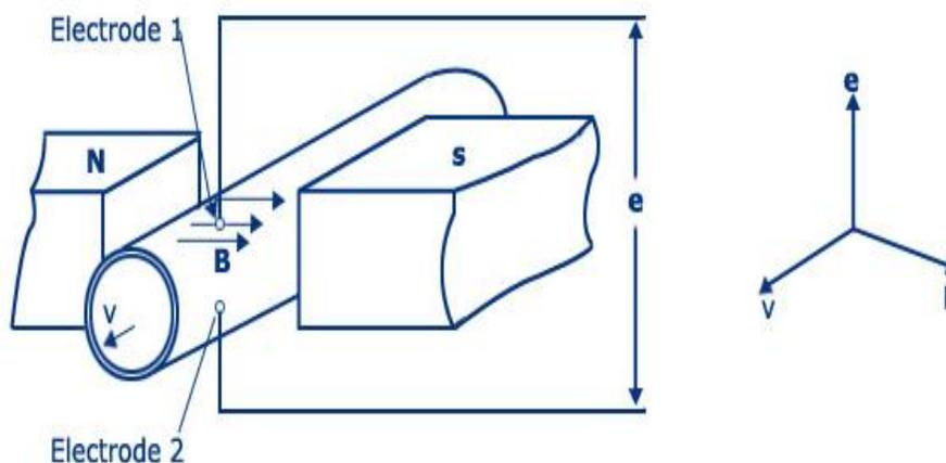
An electromagnetic flow meter can be used to measure the flow of fluids. According to Faraday's law, a voltage 'e' is induced in a conductor of length 'l' meters which is dependent on the flux density and liquid flowing velocity 'v'm/s. The parameter used for the measurement of flow is the speed of flow, and is measured in terms of the potential difference induced when the moves in a tubing/pipe with a transverse magnetic field impressed.
