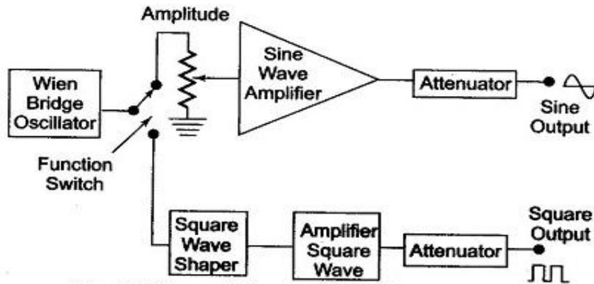
Fig. AF Sine and Square Wave Generator
