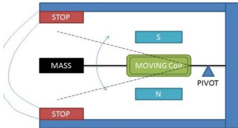
A voltage is generated on account of motion of the coil in the magnetic field. The output voltage is proportional to the velocity.
