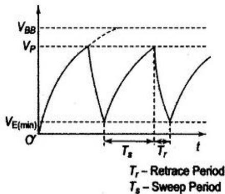
It is necessary that horizontal deflection starts at the same point of the input vertical signal, each time it sweeps. Hence to synchronize horizontal deflection with vertical deflection a synchronizing or triggering circuit is used. It converts the incoming signal into the triggering pulses, which are used for the synchronization.
