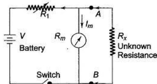
Fig. 4.30 Shunt Type Ohmmeter
